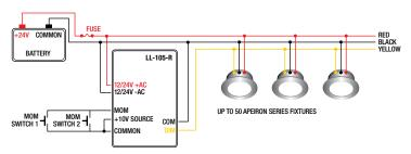
**NOTE:** MOM Switch 2 is optional. Add switches in parallel to increase the number of user interfaces for 1 LightLink.
